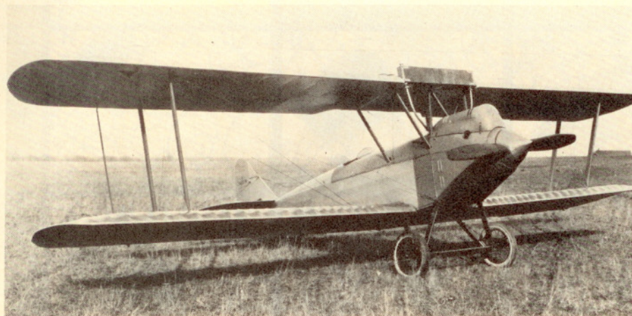
The prototype Swallow mailplane was essentially the 90-hp three-seater with slightly longer wings and a 160-hp Curtiss C-6 engine. After initial tests, the radiator was relocated from the center section to the belly, and a fuel tank was added to the center section. The use of straight-axle landing gear, after the divided-axle type on the 90-hp model, seems a step backward.
