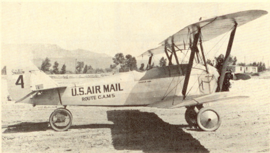
The water-cooled Curtiss engine was unsuitable for Varney's desert operation, and the fleet was grounded while new 200-hp Wright J-4, air-cooled, radial engines were installed. Pilot Franklin Rose, whose name appears on the side of No. 4, later became a fixed-base operator at Alameda, Calif.
